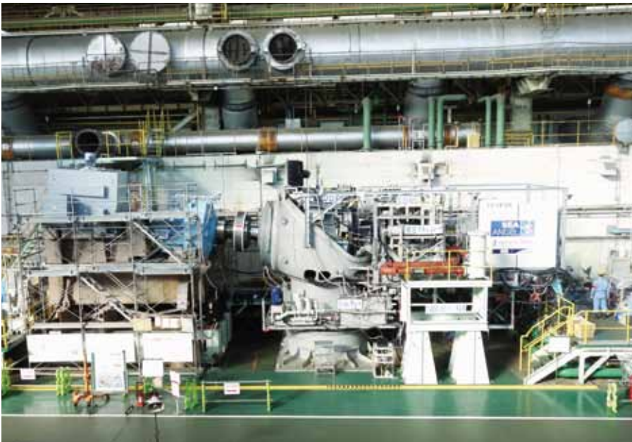
Hydraulic DDT nacelle was loaded to 2.4MW class wind turbine tower top after shop test (Top) Hydraulic DDT nacelle shop test. (Right) Transportation from test shop to wind turbine test site and power generation test of 2.4MW class wind turbine
