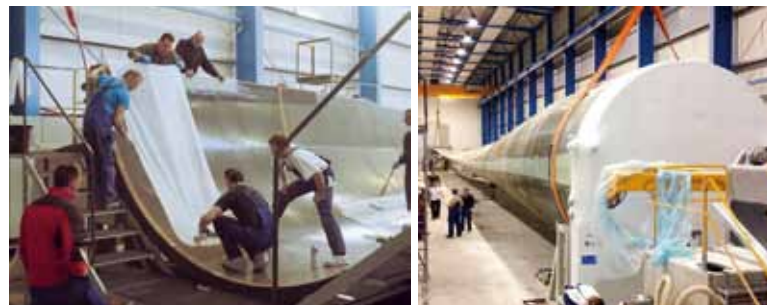
Manufacture of the first blade (Left) Moulding work of the first blade at blade manufacturing shop (Right) Complete moulding of the first blade of 81.6m length
