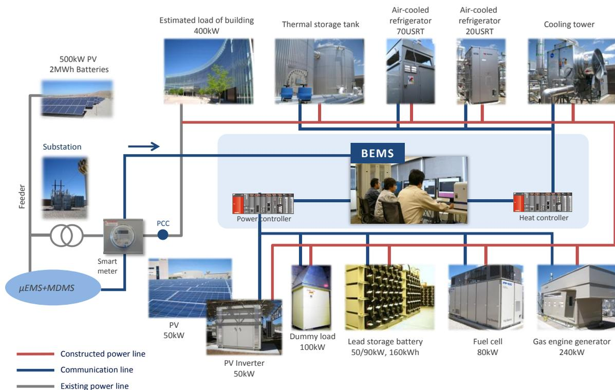
Figure 3 BEMS configuration
