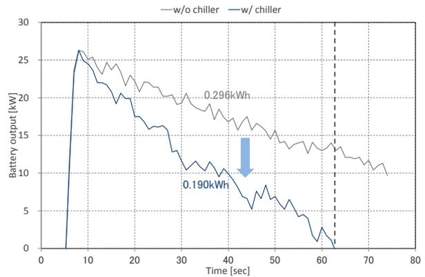
Figure 8 Effect of BESS capacity reduction due to integration of refrigerator to BEMS
