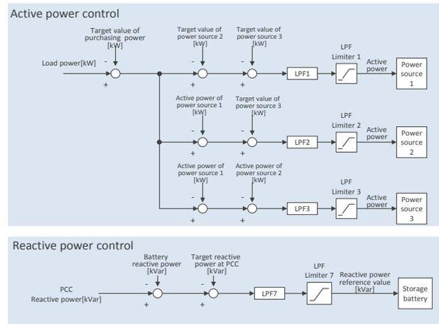
Figure 4 Control method for grid-connected mode
