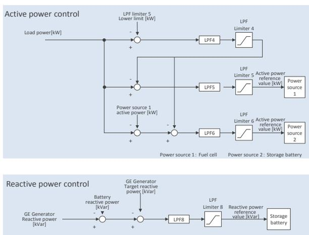
Figure 6 Control method for islanding mode
