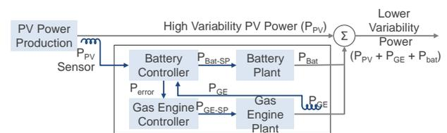
Figure 12 Coordinated Control of gas engine and battery
