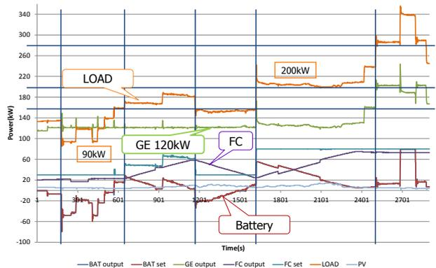
Figure 16 Results of islanding operation of Tokyo Gas' BEMS2
