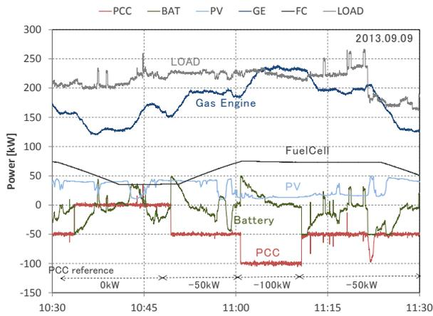
Figure 5 Performance results in grid-connected mode
