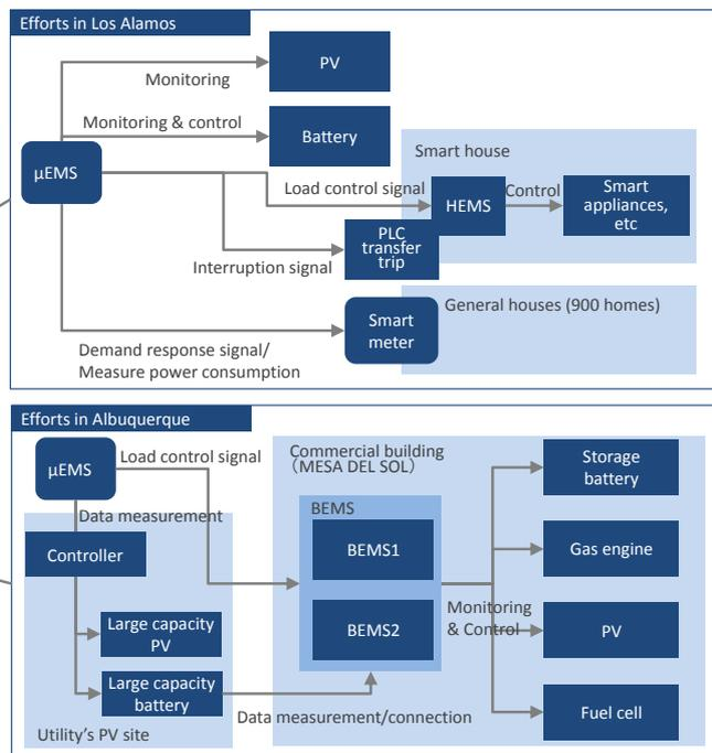
Figure 1 Whole picture of Japan-U.S. Collaborative Smart Grid Demonstration project in New Mexico
