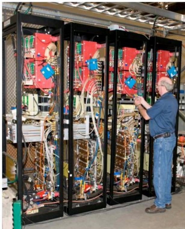
図 5.3.1-1 開発した 1MVA 級 SST (© 2011 IEEE. Reprinted, with permission, from Mrinal K. Das; Craig Capell; David E. Grider; Scott Leslie; John Ostop; Ravi Raju; Michael Schutten; Jeffrey Nasadoski; Allen Hefner: “10 kV, 120 A SiC half H-bridge power MOSFET modules suitable for high frequency, medium voltage applications”, Proceedings of 2011 IEEE Energy Conversion Congress and Exposition, pp. 2689 – 2692, 2011)
