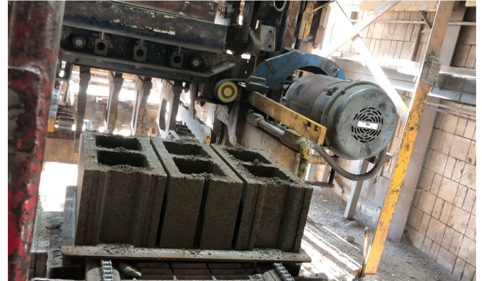
CarbonBuilt concrete blocks coming off of the production line. Each CarbonBuilt concrete block stores about three-quarters of a pound of carbon dioxide.
