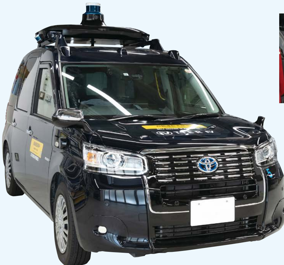
In addition to an Autoware controlled system, this experimental vehicle is equipped with 14 LiDAR devices and cameras, a global navigation satellite system, and an inertial measurement unit.
