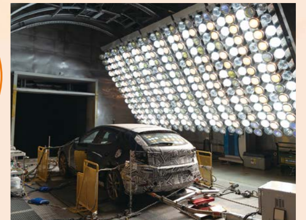
Wind tunnel test facility for vehicles that can reproduce ambient temperatures from -40 to 55 degrees Celsius and humidity conditions from 30 to 100%
