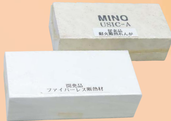
External view of conventional insulator (upper right) and newly developed insulator (lower left) While conventional insulators weigh 2.9 kilograms, newly developed ultra-lightweight insulator weighs just 370 grams
