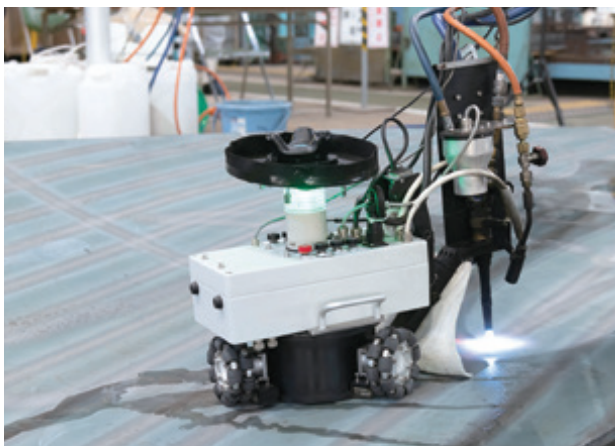
Self-propelled AI linear heating robot under development, with up to four robots working together.
