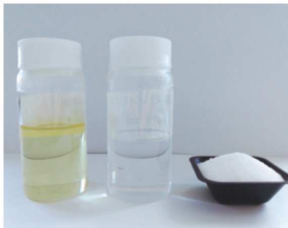
Decomposed oil (left) recovered monomer styrene (center), and recycled polystyrene (right).
