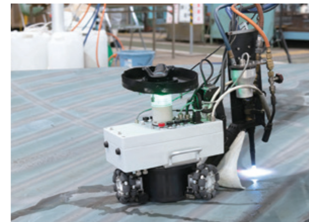
Self-propelled AI linear heating robot under development, with up to four robots working together.
