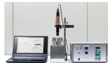
超微量粘度計 (RSM-MV1) (Ultra-trace viscometer)
