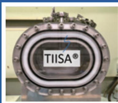
TIISA®, a super-insulating packing material for liquid hydrogen storage containers (left) Super-insulating TIISA® to prevent flames at 1300°C (right)
