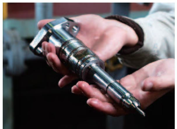
Pilot fuel injection valve for ignition - one of the key components that have made it possible to achieve the high efficiency.
