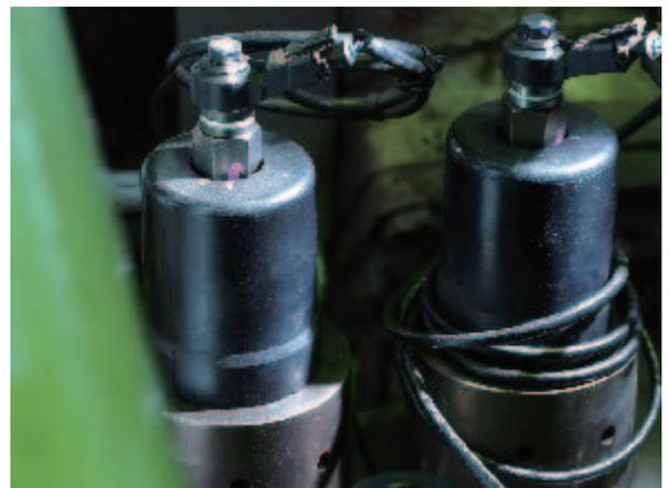
Knocking detection sensor attached to the gas engine
