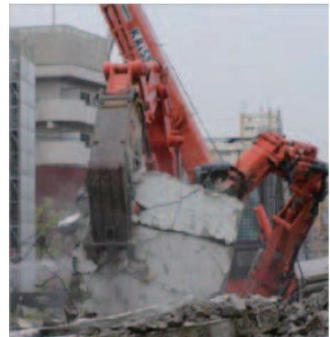
In a dual-arm machine where one arm crushes or excavates while the other arm supports, the loads on each of the arms greatly differ. (photo taken of a prototype)
