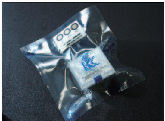
Very delicate crystal, packed for delivery to avoid exposure to air
