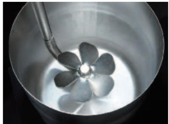
Heated, stirred melting pot used with solution stirring method
