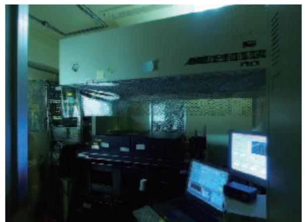
Deep ultra violet laser diffraction pitch calibration system at Japan Quality Assurance Organization (JQA)
