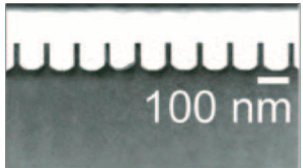
Cross sectional microscope image of ultra-fine scale at 100nm intervals
