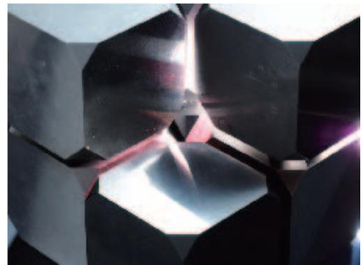
Inside the multi-anvil developed by Sumiya at Sumitomo Electric Industries, Ltd. for mass production of artificial diamonds
