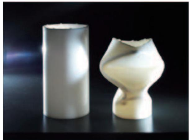
As a result of a destruction test, a conventional product cracked while the impact absorbing nylon was only dented like an empty can. Recovery from this state is also possible.
