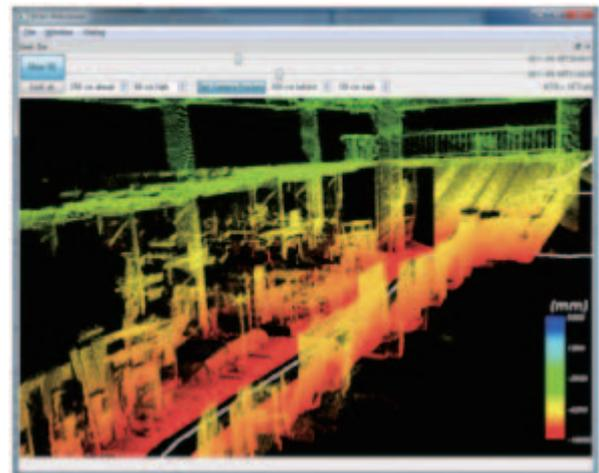
Image of the inside of a campus building of the Chiba Institute of Technology recorded by “Quince” with a laser scanner (image courtesy of Chiba Institute of Technology fuRO)
