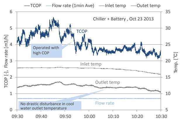
Figure 9 TCOP and cold water outlet temperature of the refrigerator which is integrated and controlled
