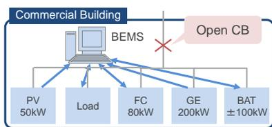
Figure 11 BEMS2 Configuration – Interconnected Operation-
