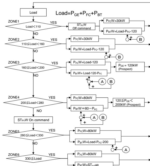
Figure 15 Logic of islanding operation of Tokyo Gas' BEMS2
