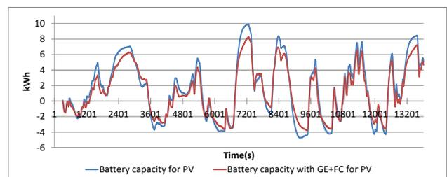
Figure 14 Verification of battery capacity reducing effect based on actual data
