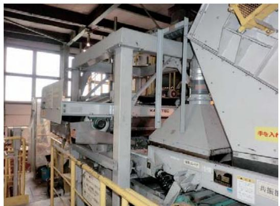
Magnetic separator that sorts out iron using magnetic force (Photo courtesy of Tokyo Eco Recycle Co., Ltd.)
