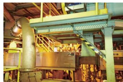
Inside the APR plant, pulverized waste plastic is pushed out of a pipe
