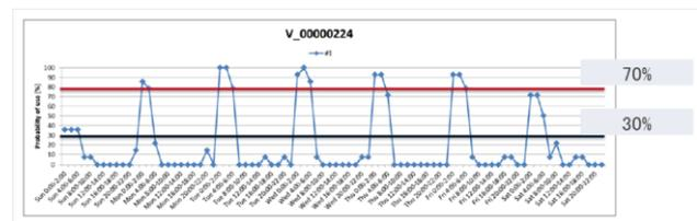
Figure 14 Probability profile of use of EV charger
