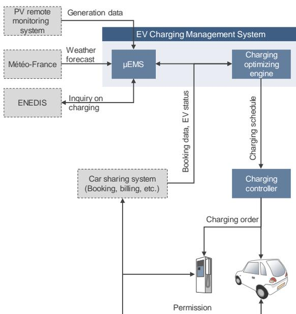
Figure 10 Overall structure of the system developed in Task2
