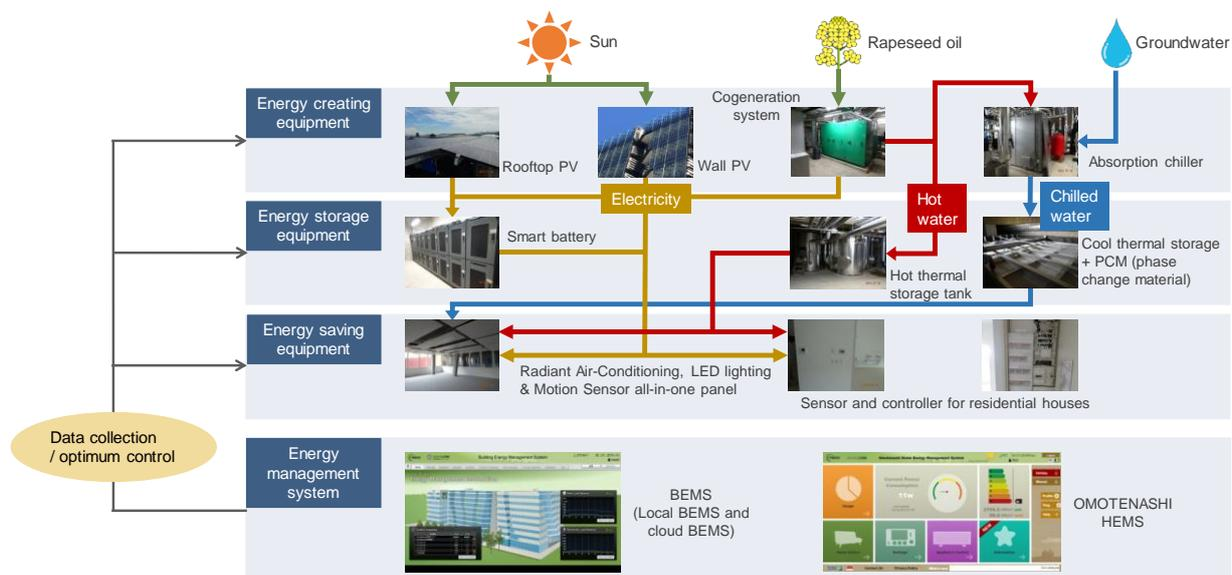
Figure 5 Task1 Structure of demonstration system
