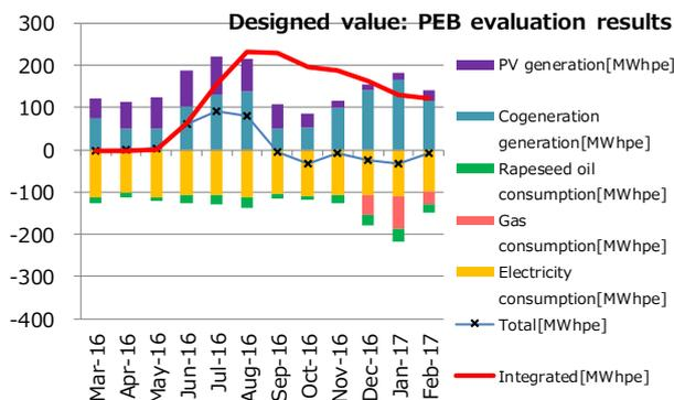
Figure 6 Annual energy balance simulation (during design)
