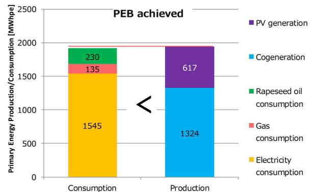
Figure 8 Result of PEB verification (after office system calibration)
