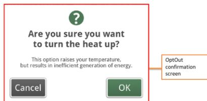
Figure 14 Display screen for Opt-Out from DR control
