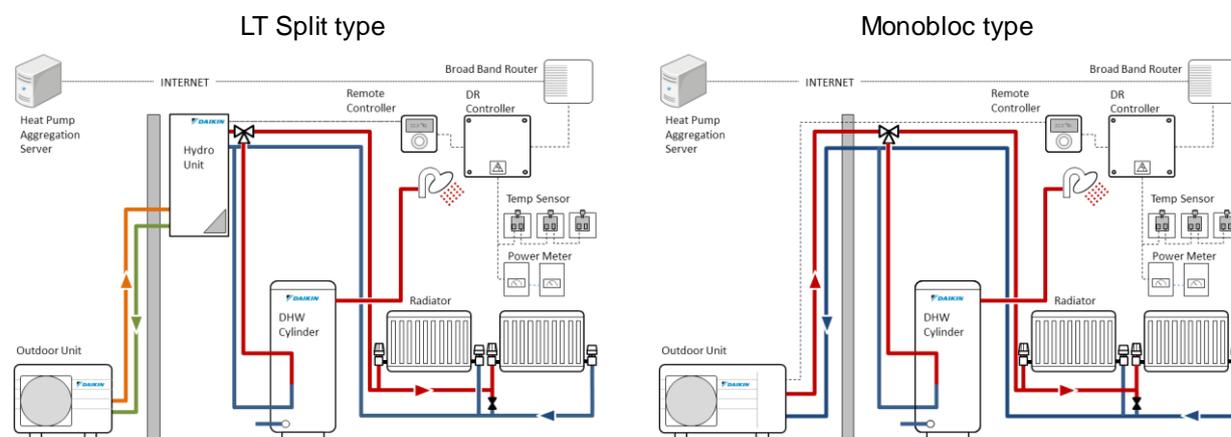
Figure 4 System configuration for LT Split type / Monoblock type
