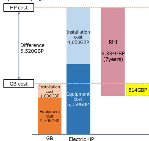
Figure 17 Comparison of introduction cost with gas boiler (Electric HP)
