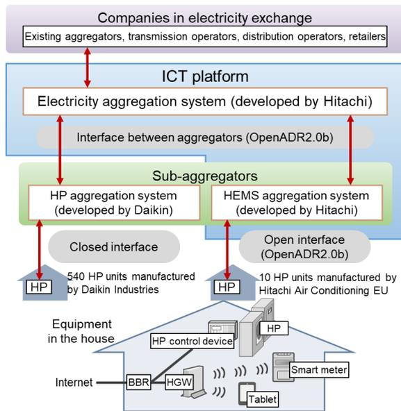
Figure 10 Overall picture of aggregation system
