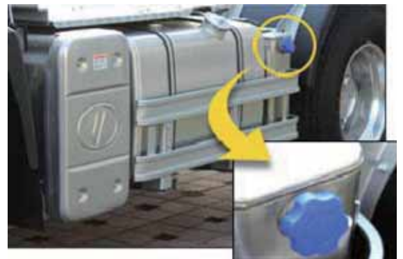
AdBlue™ tank next to a diesel fuel tank The color and size of the AdBlue™ tank filler caps differ from those of diesel fuel tank fillers.
