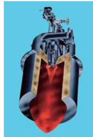
High-load combustion (vortex burner)
