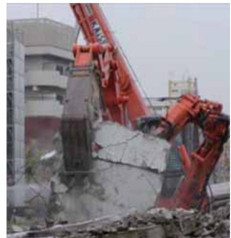
In a dual-arm machine where one arm crushes or excavates while the other arm supports, the loads on each of the arms greatly differ. (photo taken of a prototype)
