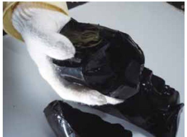
Melted and neutralized asbestos
