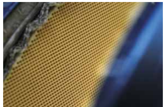
Interior of the reduction unit The mesh structure increases the contact area and improves reaction efficiency. NOx is removed at the surface of the mesh structure.
