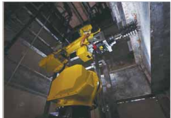
Asbestos-removal robot designed for use in an elevator shaft
