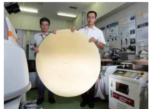
Large epoxy grinding pad with a diameter of 1200mm (Professor Tani (left) and Mr. Nomura, head of the development staff of KOKONOE ELECTRIC CO.,LTD. (right))
