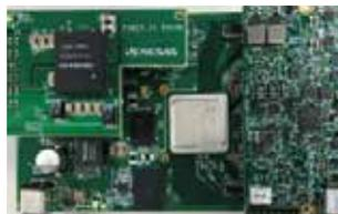
AI system board equipped with DRP-AI chip for vision-AI processing with high accuracy and low power consumption
