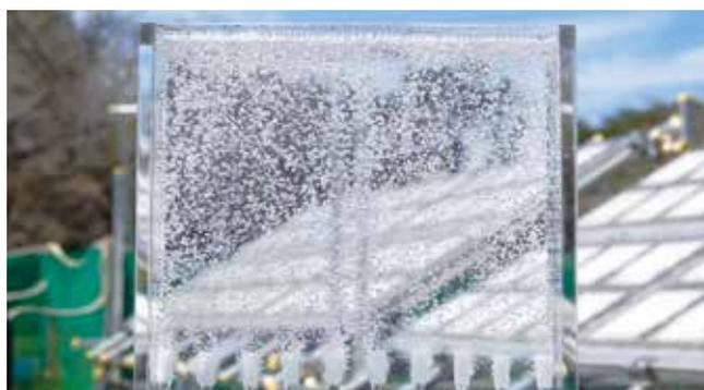
Gas mixture of hydrogen and oxygen generated from photocatalytic panel reactor
