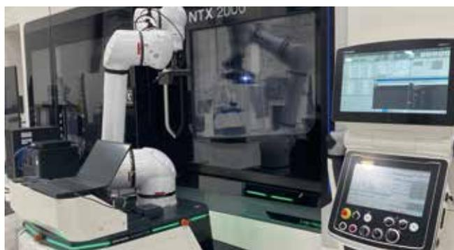
A multi-skilled self-propelled robot with processing assist function
