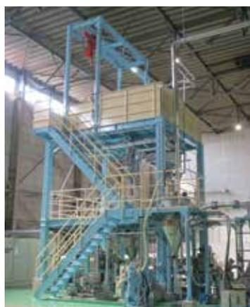
CNF-reinforced resin kneading extruder
