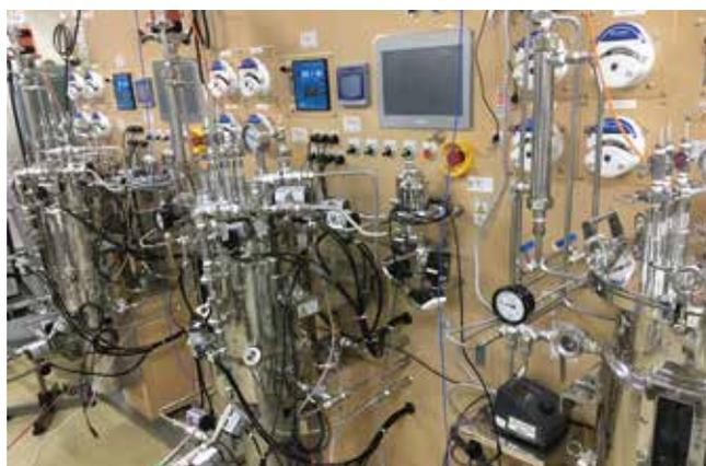
30L-scale fermentation systems used for validation of practical applications and development of bio-manufacturing processes
