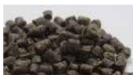
CNF-reinforced resin (Cellenpia Plas<sup>®</sup>) masterbatch pellets
