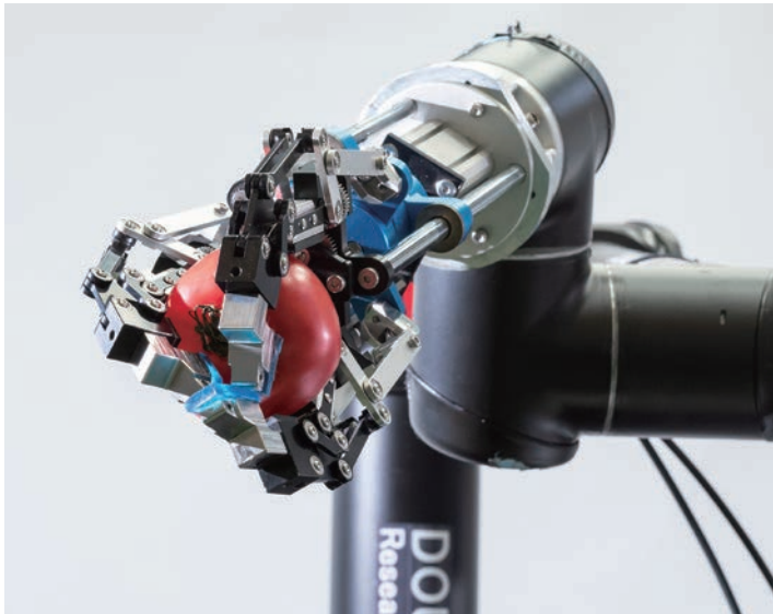
D-Hand Type R, a three-finger robotic hand featuring a locking mechanism, has improved the performance of grasping and pinching functions compared to the previous model (left). The D-Hand, a five-finger model equipped with seven motors that enable movements more similar to those of a human hand, can lift soft objects, such as cream puffs, without crushing them, as it is better able to control the motor output (right). (Source: Double Giken Co., LTD.)
