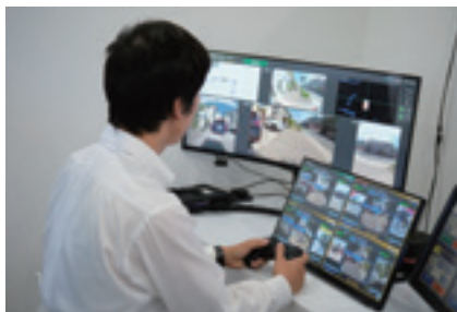
Four HAKOBO robots are remotely operated by a single operator (Source: Panasonic Holdings Corporation)
