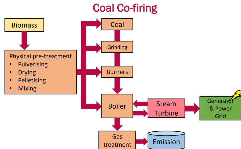
Flowchart of the Coal Co-firing process
