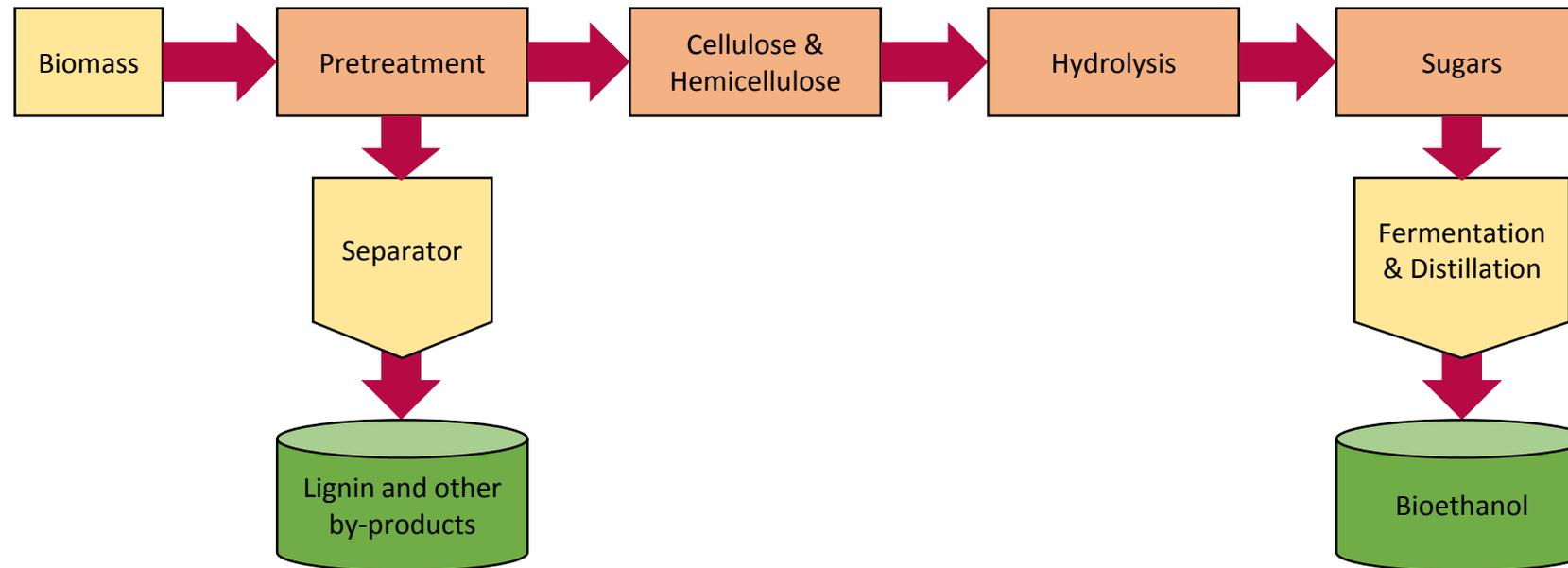
Schematic representation of production of bioethanol from cellulosic biomass
