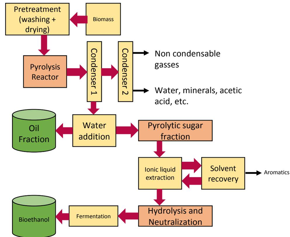
Flowchart of bioethanol production via the pyrolysis process
