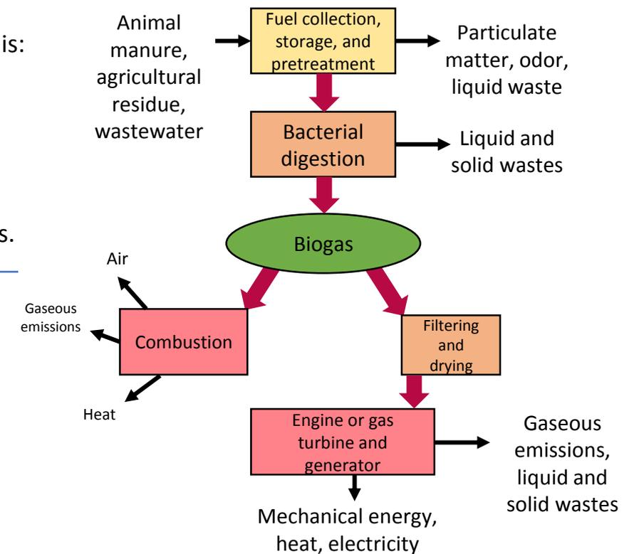
Flowchart of biogas production via the anaerobic digestion process
