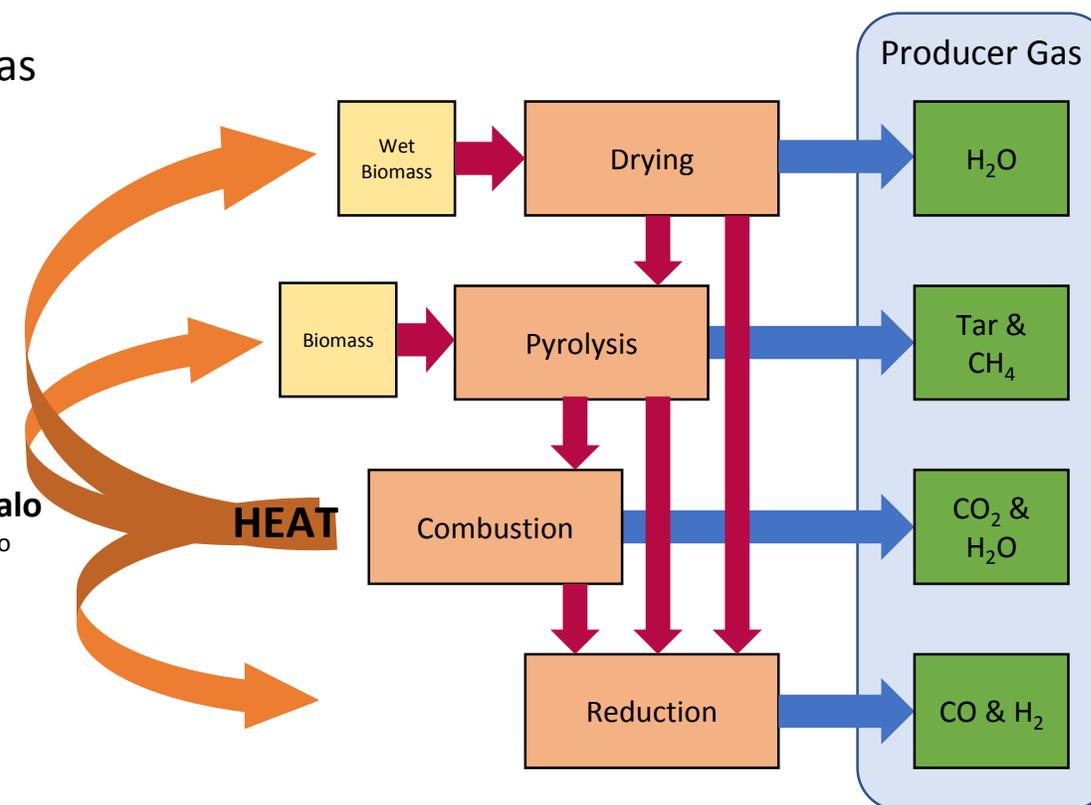
Schematic representation of biomass gasification
