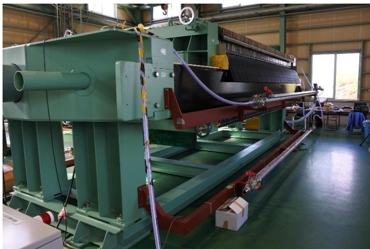
Half-set electrolyzer test for Fukushima project
