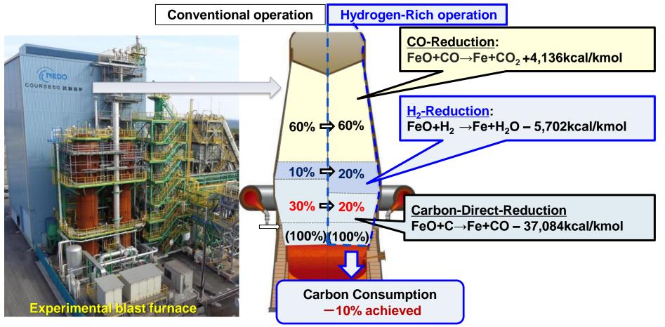
In the experimental blast furnace, 10% reduction in carbon consumption has been achieved by hydrogen-rich operation.
