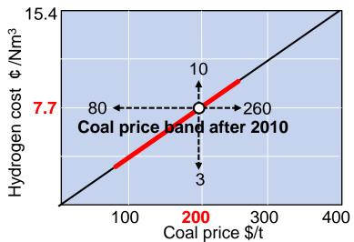
A trial calculation : Assuming **\$200/t-coal** and **700kg-coal/t**-hot metal, coal cost is **140\$/t**-hot metal.
