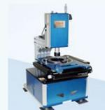
The XS-1Sirius crystal dislocation visualization equipment with a dislocation counting system and heat map display function
