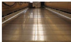
A passenger cabin floor panel of Shinkansen using flame-retardant magnesium alloys
