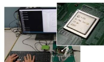
Evaluation chips and evaluation boards for design and evaluation platform of proprietary IP for AI chips
