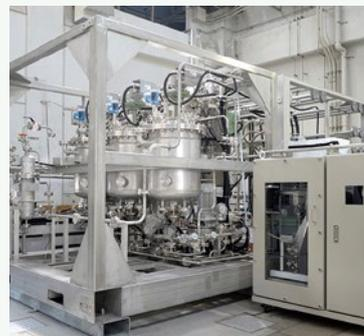
The iFactory<sup>®</sup> module (left) and automatic analysis device (right)
