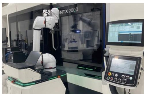
Multi-skilled self-propelled robot with processing assist functions
