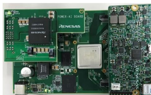
AI system board mounted with DRP-AI chips
