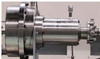
The stand-alone ORC power generation system (5 kW class) incorporating a scroll-type expander (above) for demonstration tests
