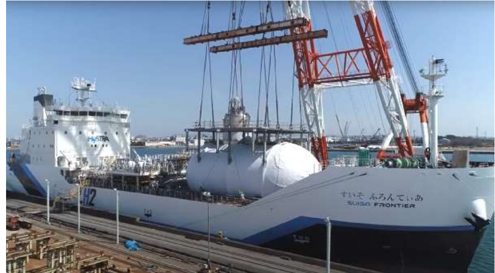
Cargo Tank Installation (7 March 2020) at KHI Harima Works
