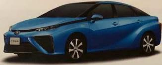
The Mirai is a fuel cell vehicle (FCV) which uses hydrogen as energy to generate electricity and power the vehicle.
