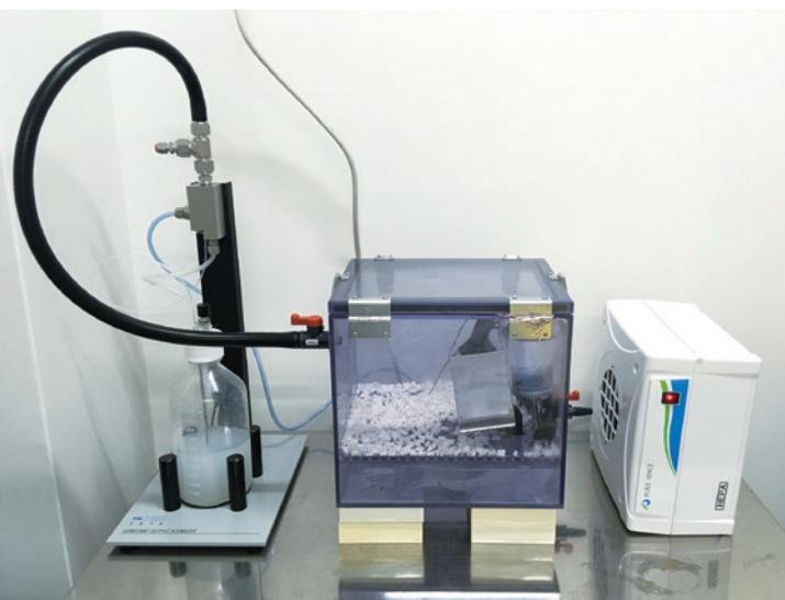
Equipment to measure level of exposure to CNF dust generated in typical workplace environment and assess impacts on inhalation.
