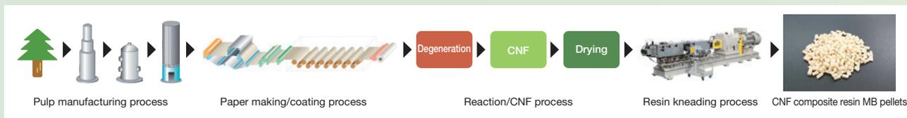
Solving various problems by improving productivity at each stage of the integrated manufacturing process, from CNF raw materials to CNF composite resin materials.
