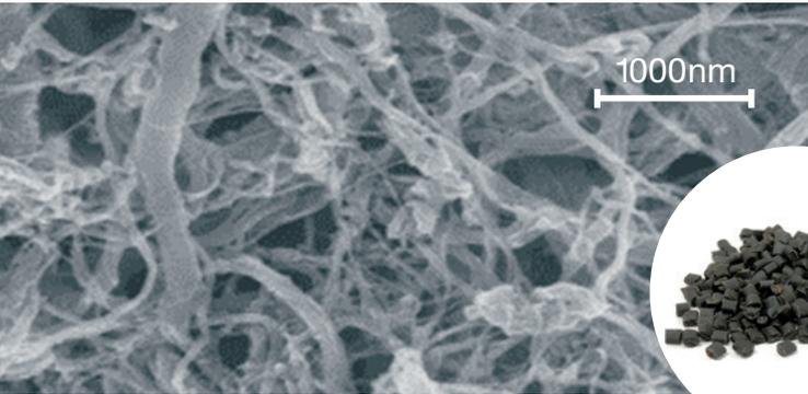
Cellulose nanofibers in CNF-reinforced resin
