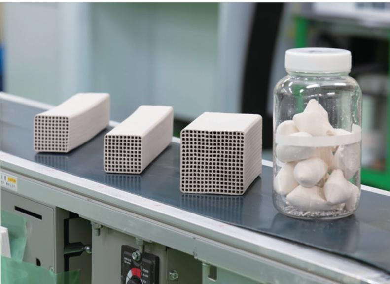
Filter elements being prototyped. Based on evaluations of CNF characteristics, research on filter shapes is progressing.
