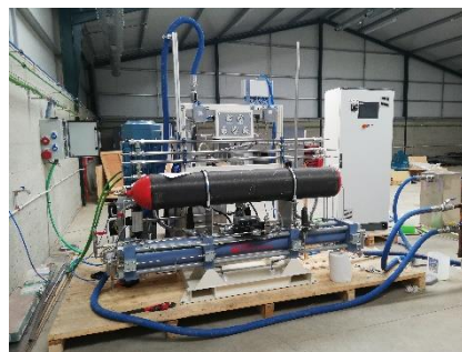
Compressor 50m 3 /h p_{in} :10-40 bar p_{out} : 300-450 bar
