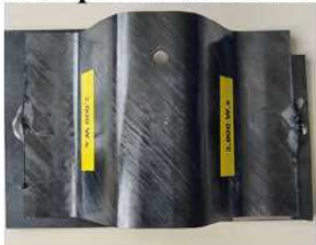
An demonstration of jig-less end-effector stringer-to-skin ultrasonic welding process.
