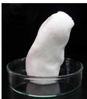
図Ⅲ-2.1.7-2 10 wt% CNF水分散液
