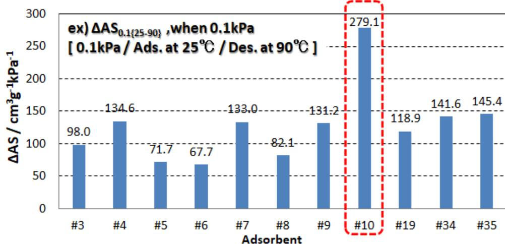
Example of adsorbent selection result using  $\Delta AS$  value (original definition)
