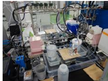
Lab. Continuous Evaluation Test Equipment for CO 2 Electrochemical Reduction
