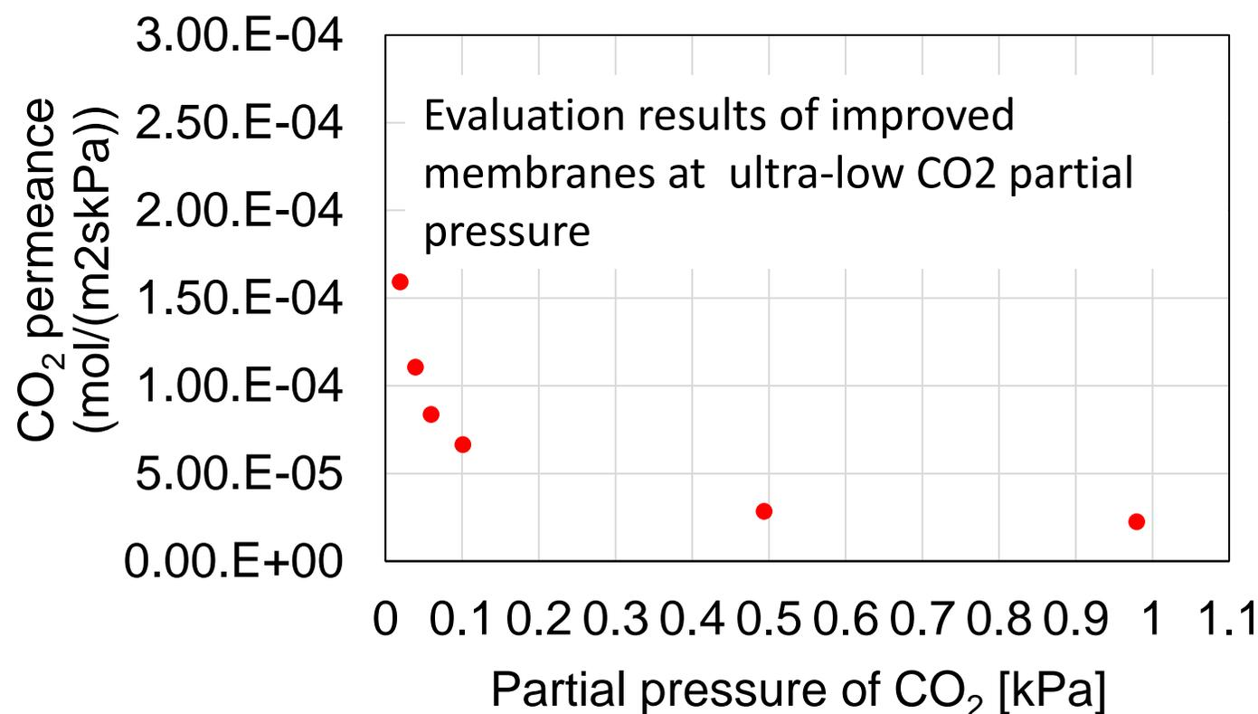
Focusing on the fact that the dependence on CO<sub>2</sub> partial pressure differs depending on the type of CO<sub>2</sub> carriers and composition of those and additives, we investigated the improvement of the performance of DAC under ultra-low CO<sub>2</sub> partial pressure conditions.
