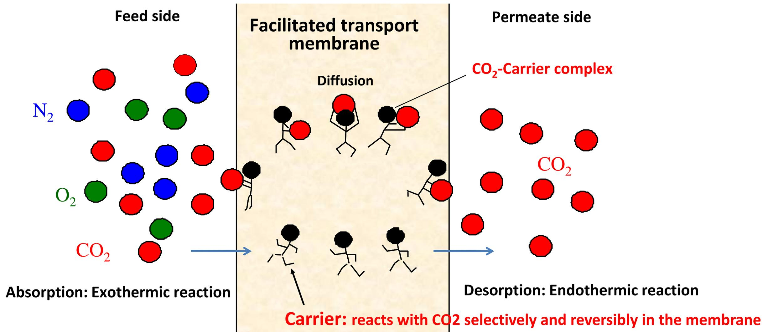
Energy required for CO<sub>2</sub> desorption can be supplied from that of CO<sub>2</sub> absorption
