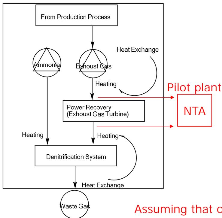
Assuming that one of the exhaust gases is extracted by side flow
