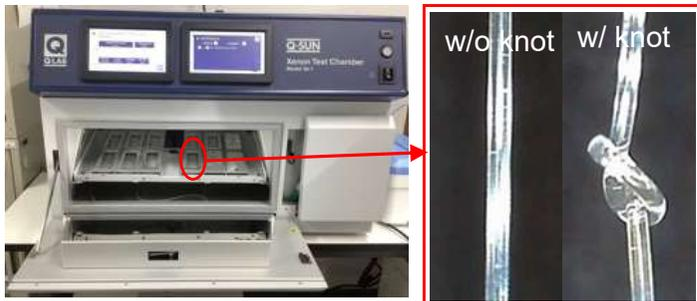
Fishing lines were UV aged by an accelerated weathering machine with total irradiance ca. 300 MJ/m<sup>2</sup> (300-400nm), which is equal to 1 year's irradiation in Choshi. Fibers with knot were employed to simulate the degradation of fishing nets.
