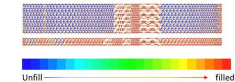
Optimization of octa-screw kneading process and CAE flow analysis
