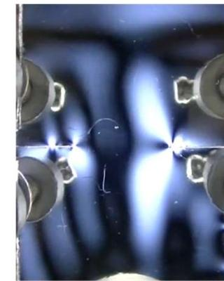
The higher the molecular weight PC showed the wider range of plastic deformation. It means large energy dissipation.
