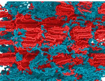
Classification of crystal and melting parts using machine learning on the results of heat degradation simulation. (Red : crystal part, blue : melting part)
