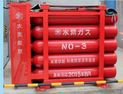
Cylinder Cardle → Crane truck
