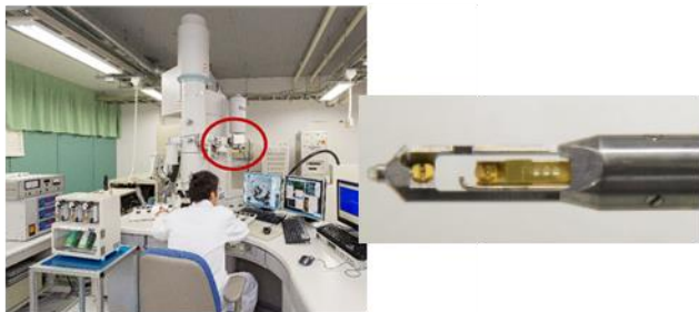
Catalyst samples could be heated up to 1500 °C in various gas atmospheres
