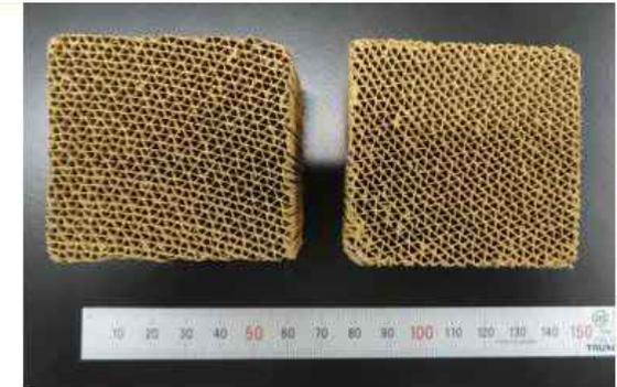
test pieces of “Honeycomb” NO adsorbent (Pd-zeolite)
