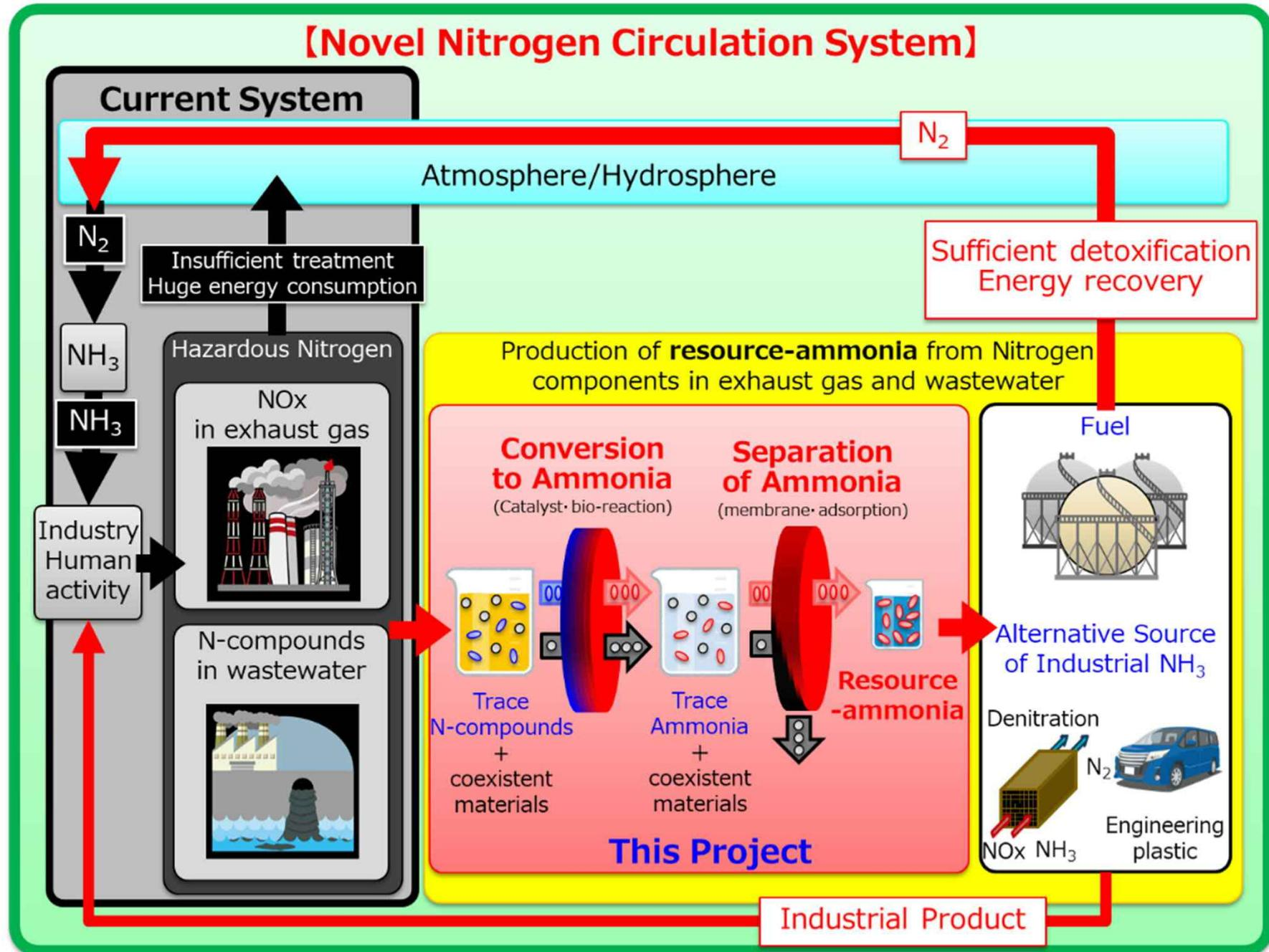
NOx in exhaust gas is converted to NH<sub>3</sub>, which is used as denitration material and industrial raw material. Nitrogen compounds in wastewater are recovered as ammonia resources and used as fuel and raw materials.
