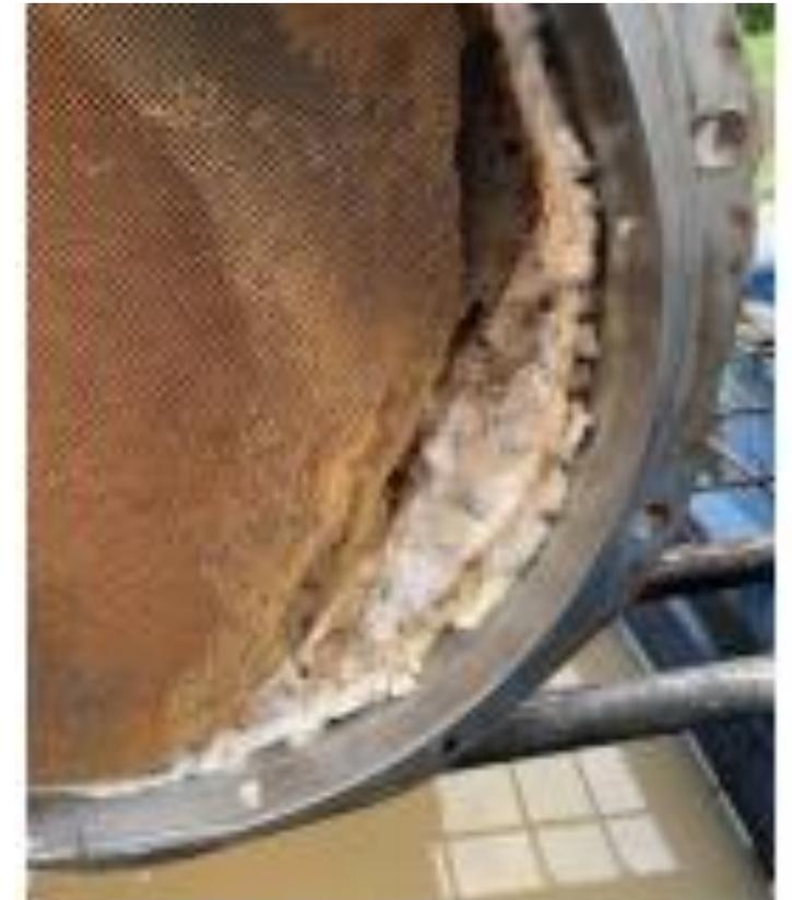
broken catalyst in NH<sub>3</sub>-SCR (by urea water)
