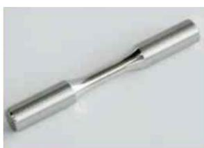
Fatigue tests (>10 cycles, 25 years operation) in liquid nitrogen proved SUS 304 to be a candidate material for the sublimation tank
