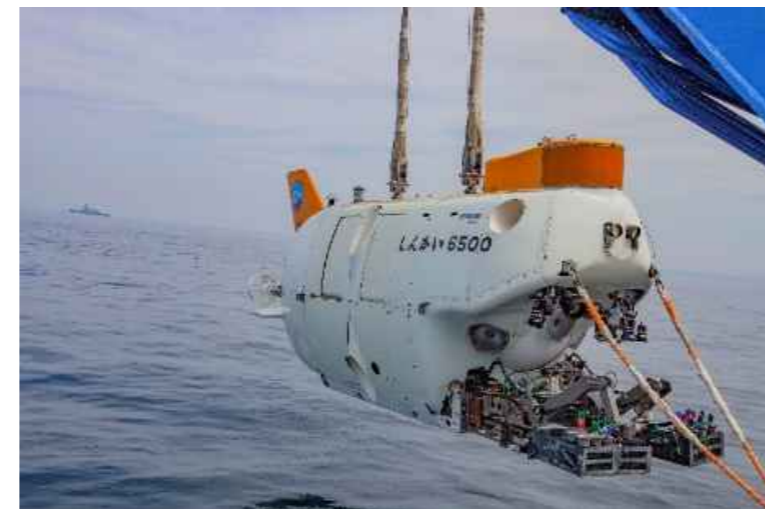
Deployment and recovery with the manned submersible
