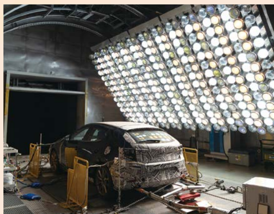
Wind tunnel test facility for vehicles that can reproduce ambient temperatures from -40 to 55 degrees Celsius and humidity conditions from 30 to 100%
